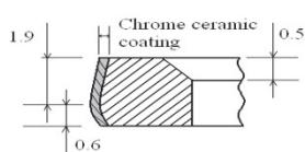
**Figure 1. Cross Sectional view of modification done to Top ring**
