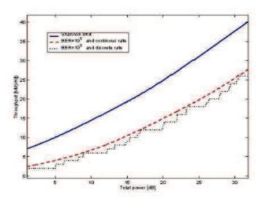
The figure above shows the data throughput (bit/(sHz)) as a function of total transmits power for a 4 times 4 MIMO system in a Rayleigh fading channel. The blue curve is the Shannon limit and the dashed curve the throughput of the BER is fixed at the target 10<sup>-5</sup>. In practice, the data rates chosen for the subchannels cannot be arbitrarily chosen, they must
