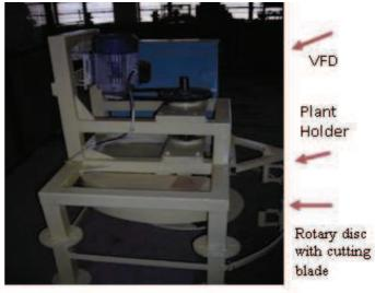
Plate.2 Experimental Set up
